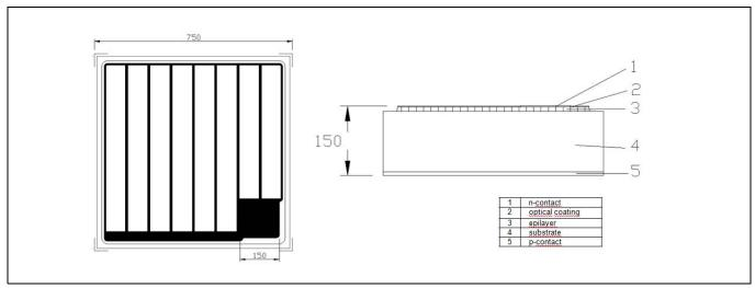
Dimensions are specified as typical 1) values as follows: µm
