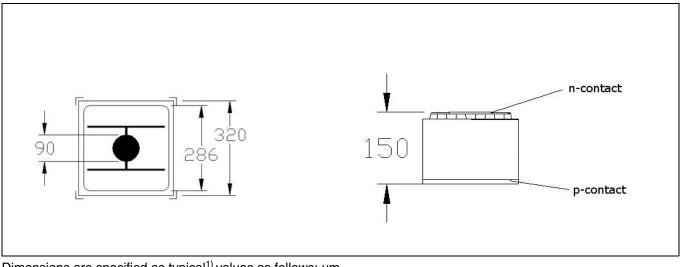
Dimensions are specified as typical  $^{1)}\,values$  as follows:  $\mu m.$
